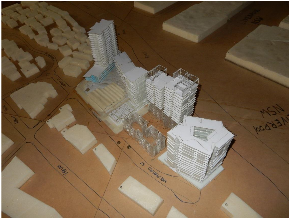
Figure 5 – View from the southwest of the scale model of the 26-28 Shepherd Street Development in the wind tunnel.
