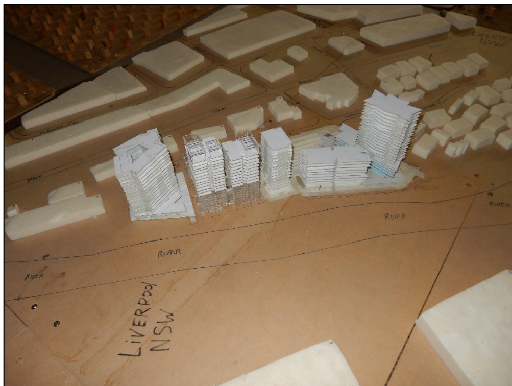
Figure 6 – View from the east of the scale model of the 26-28 Shepherd Street Development in the wind tunnel.
